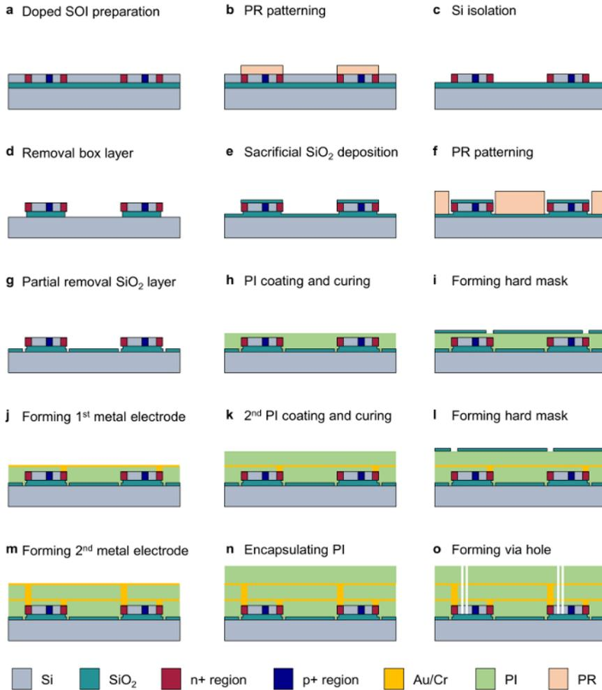
**Figure 1: Schematic illustrations of the fabrication process of the curved phototransistor array.** The panels (a) - (o) show the sequential process from fabricating a phototransistor device on a doped SOI substrate to creating a via hole to remove the sacrificial layer of the SOI substrate. [Please click here to view a larger version of this figure.](#)
