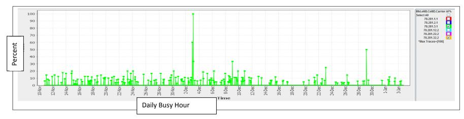
KPI access failure rate demonstrates over 2% for the entire time period reflected. Access failures as high as 60% were recorded.
