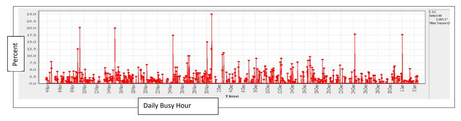
KPI access failure rate demonstrates over 2% for the entire time period reflected. Access failures as high as 25% were recorded.
