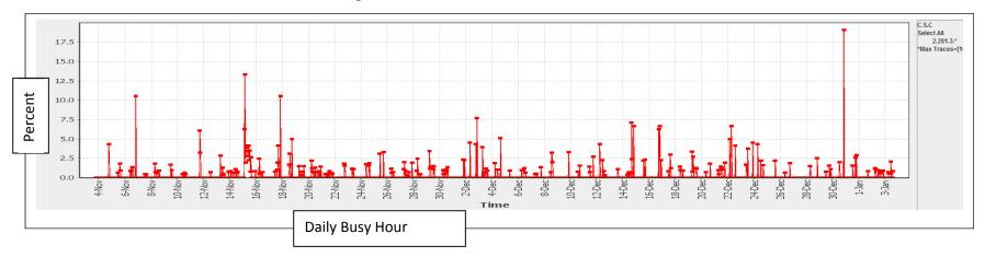
KPI Drop Call rate demonstrates over 1% for most of the time period reflected. Drop Calls as high as 17% were recorded.
