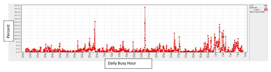
KPI access failure rate demonstrates over 2% for a majority of the time period reflected. Access failures as high as 32% were recorded.
