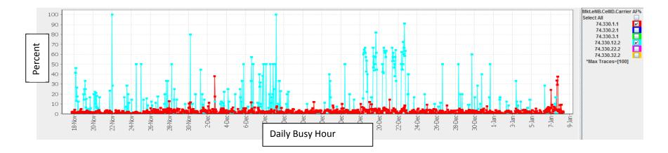
KPI access failure rate demonstrates over 2% for a majority of the time period reflected.
