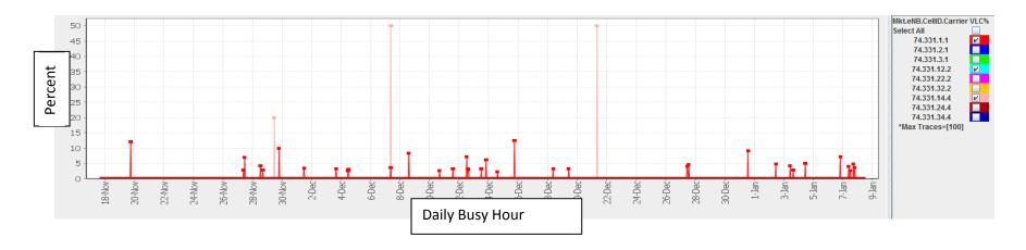
KPI Drop failure rate demonstrates over 1% for a majority of the time period reflected.
