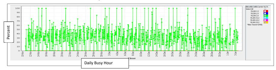
KPI Drop failure rate demonstrates over 1% for the entire time period reflected. Drop failures as high as 100% were recorded.
