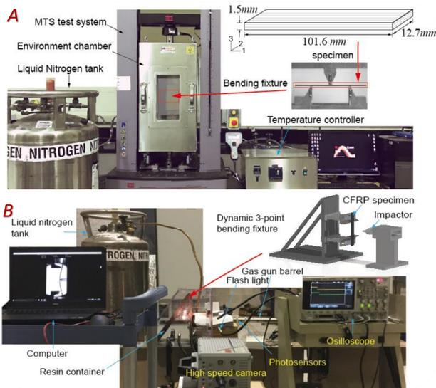
Figure 1. (A) Static and (B) dynamic three-point bending experiment setup. Specimen size is shown in upper right of A.
