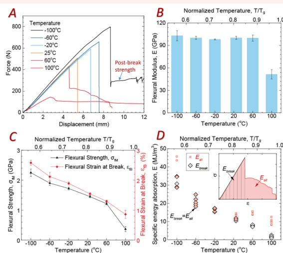
Figure 2. Static 3-point bending results at various temperatures: (A) force displacement curves, (B) flexural modulus, (C) flexural strength and flexural strain at break, and (D) energy absorption per volume.
