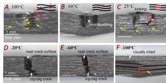
Figure 3. Post mortem photographs. (a) Extension mode microbuckling. (b) Shear mode microbuckling. (c) Kink band and inter-fiber cracks. (d, e) Catastrophic damage. (f) Inter-fiber cracking at bottom layer.
