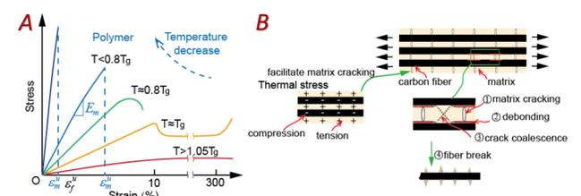
Figure 7. Temperature effect origin. (A) Temperature dependency of polymer. (B) Thermal stress effect, and typical cracking process of brittle matrix CFRP.
