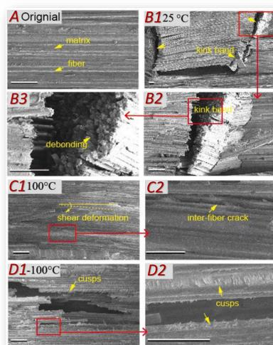
Figure 4. SEM image of the rectangular regions in Fig.3. (A) original specimen, & specimens at (B1-B3) 25°C, (C1-C2) 100°C, and (D1-D2) -100°C.
