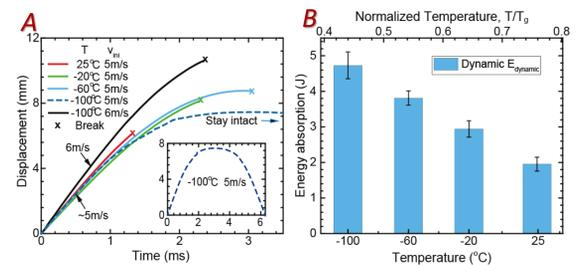
Figure 5. Dynamic 3-point bending results. (A) Displacement history, and (B) energy absorption at 25°C, -20°C, -60°C and -100°C.
