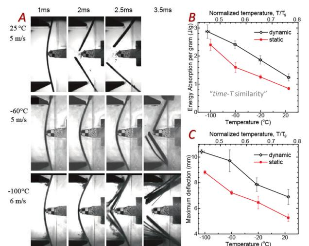
Figure 6. (A) Dynamic deformation of CFRP at different moments. Comparison between static and dynamic 3-point bending results: (B) energy absorption per gram, (C) maximum deflection at break.
