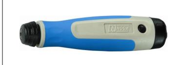
NG-2 Handle accepts all "N" type Blades Ergonomic soft grip, acetyl and rubber construction Removable end cap for blade storage 125mm long x 28mm maximum diameter Blades are secured by pulling back the front locking mechanism and are free to rotate
