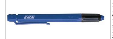
Plastic Edge Off Handle will accept all "S" type Heavy Duty Blades with 3.2mm shank Complete with moulded pocket clip Blades are secured by turning the front locking mechanism and are free to rotate Manufactured from tough ABS plastic Size 120mm long x 10mm hexagonal section
