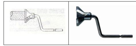
90° External Rotodrive Chamfer Head Range: 4 – 18mm diameter Blade shank diameter 3.2mm Blade material: HSS M2 Blade hardness: 62-64 HRC Used with NG-1 Handle or S Holder with NG-3 Handle
