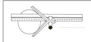
Provides centre position on diameters up to 105mm / 4 1/4"
