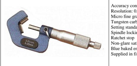
Accuracy conforms to DIN 863 Resolution: 0.01mm Micro fine graduations for accurate reading Tungsten carbide spindle and anvil faces Setting standard Spindle locking lever Ratchet stop Non-glare satin chrome barrel and sleeve Blue baked enamel hammer tone finish Supplied in fitted case with adjustment tools
