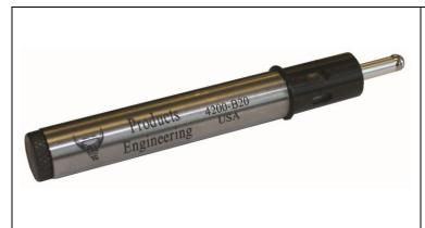
Edge Finders provide a fast and accurate method of allowing the work piece to be moved to a known position relative to the centreline of the machine spindle
