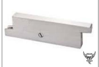
Each parallel consists of 2 pieces dovetailed together so they can slide on each other to change the height and then locked by means of hex set screws (3/32" A/F)
