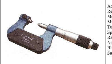
Accuracy conforms to DIN 863 Resolution: Metric 0.01mm, Models above 25mm supplied with setting rod Micro fine graduations for accurate reading Tungsten carbide measuring faces Spindle locking lever Ratchet stop Non-glare satin chrome barrel and sleeve Blue baked enamel hammer tone finish Supplied in fitted case with adjustment tools
