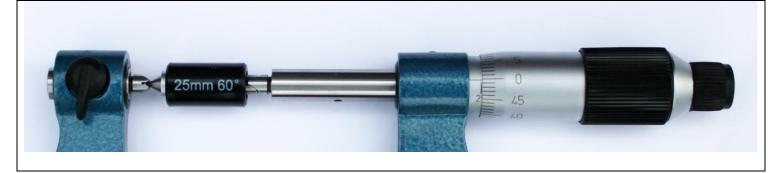
Select, clean and insert the required pair of thread elements
