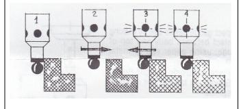
Inspect the Edge Finder before use by making contact between ball and body using a metal paper clip or steel rule
