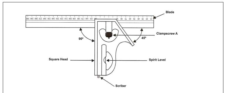
Note: Graduations are on both edges of the blade. Diagram shows only on one edge as it is intended for general information only
