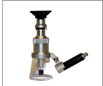
There are 4 microscopes in this range, offering the following magnifications: 25, 50, 75 & 100 Each Microscope has the following features Measuring Scale Rubber Eye Cup Focussing Ring Acrylic object surround Side mounted mini torch (batteries not included) Mini torch requires 3 x 1.5V Alkaline button cells SR44 Max. Height: 145mm Acrylic Base Diameter 45mm Supplied in a foam lined case
