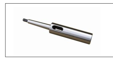
Morse Taper Extension Sleeves allow cutting tools with a Morse Taper Shank to be fitted to machine spindles which have a different Morse Taper to that of the tool. They also provide extended length to taper shank tools
