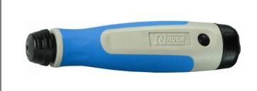
NG-2 Handle accepts all "N" type Blades Ergonomic soft grip, acetyl and rubber construction Removable end cap for blade storage 125mm long x 28mm maximum diameter Blades are secured by pulling back the front locking mechanism and are free to rotate
