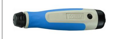
NG-1 Handle accepts all "S" type Blades Ergonomic soft grip, acetyl and rubber construction Removable end cap for blade storage 125mm long x 28mm maximum diameter Blades are secured by pulling back the front locking mechanism and are free to rotate
