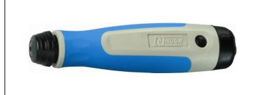
NG-1 Handle accepts all "S" type Blades Ergonomic soft grip, acetyl and rubber construction Removable end cap for blade storage 125mm long x 28mm maximum diameter Blades are secured by pulling back the front locking mechanism and are free to rotate
