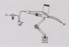
c. Setup to supply drops and air jet independently
