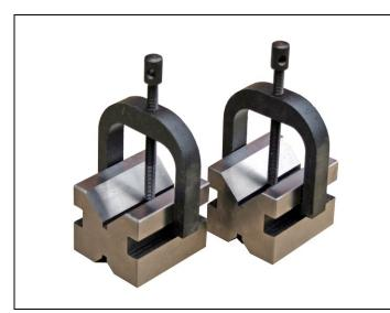
Manufactured from Carbon Steel 45# Hardness HRC 55 - 62° Supplied in matched pairs with clamps Matched Pair Accuracy: 0.005mm
