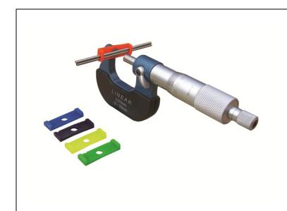
Thread Wire Attachments are suitable for holding 2 wires against the fixed micrometer anvil leaving one hand free to operate the micrometer and the other hand free to position the 3<sup>rd</sup> wire in the opposing thread groove.
