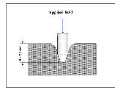
The principle used to determine Shore Hardness is based on measuring the resistance force of the penetration of an accurately ground conical probe into the test material under a known spring load The amount of penetration is converted into a Shore Hardness value on a dial with 100 Shore Hardness graduations
