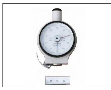
Shore Durometers provide a fast and convenient method of measuring the hardness of rubbers, plastics, leather and other soft materials
