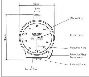
Specimen size should allow measurement to be taken at least 12mm from any edge
