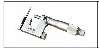
Accuracy conforms to DIN 863 Resolution: Metric 0.01mm, Inch 0.0001" Micro fine graduations for accurate reading Tungsten carbide spindle face Spindle locking lever Ratchet stop Non-glare satin chrome barrel and sleeve Satin chrome steel body Supplied in fitted case with adjustment tools
