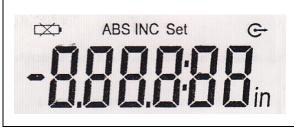
In : Inch Mode INC : Relative Measuring ABS : Absolute Measuring : Battery Voltage is Low O : Data Output Set : Set the Origin Hold : Display value Held
