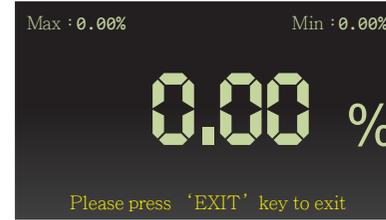
Enter Duty/Cycle (%) and connect positive probe (Red) with sensor and the negative probe (Black) with chassis ground of the vehicle in order to measure the percentage.
