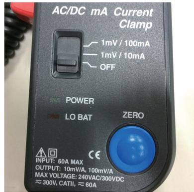
Please select proper condition for the Current clamp measurement, for example in order to measure 1mV=0.01A with CA15, move the switch to the 1mV/10mA on Current clamp.
