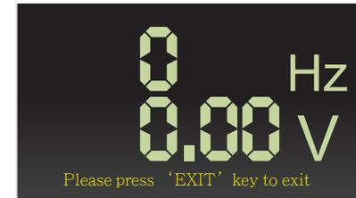
Enter CAM/CRANK/SPEED Sensor and connect positive probe (Red) with sensor and the negative probe (Black) with chassis ground of the vehicle in order to perform measurement.
