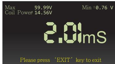
Enter Injection System to select display mode: Injection Time Scanwaveform (waveform).
