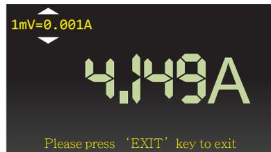
In order to measure the Current accurately press the ZERO button on the current before performing the measurement.
