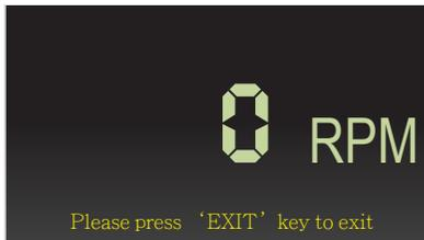
Enter RPM and connect positive probe (Red) with sensor and the negative probe (Black) with chassis ground of the vehicle in order to perform measurement.
