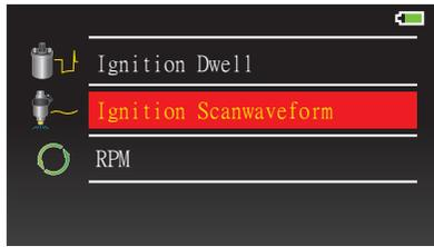
Confirm Ignition type and number of cylinders when entering to measure Ignition Dwell Angle.
