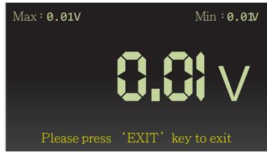
Enter O2 Sensor and connect positive probe (Red) with sensor and the negative probe (Black) with chassis ground of the vehicle in order to measure O2 Sensor Voltage.
