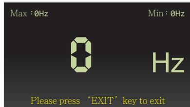
Enter Frequency (Hz) and connect positive probe (Red) with sensor and the negative probe (Black) with chassis ground of the vehicle in order to measure frequency.
