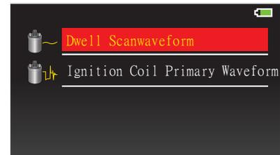
Enter Ignition Primary to select Dwell Scanwaveform or Ignition Coil Primary Waveform.
