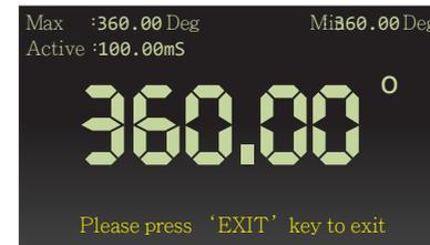
Enter Ignition Dwell and connect positive probe (Red) with sensor and the negative probe (Black) with chassis ground of the vehicle in order to perform measurement.
