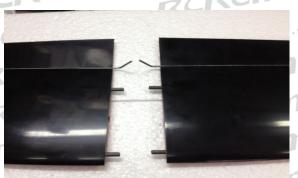
• Use the hardware provided by the ARF kit...fix the iron stick like you see in the picture and glue it using epoxy.
