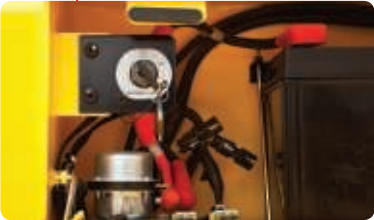
Master Switch A master switch disconnects the battery power to protect the electrical system from excess electrical drainage.
