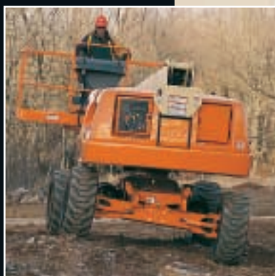
Oscillating Axle for Tough Travel
