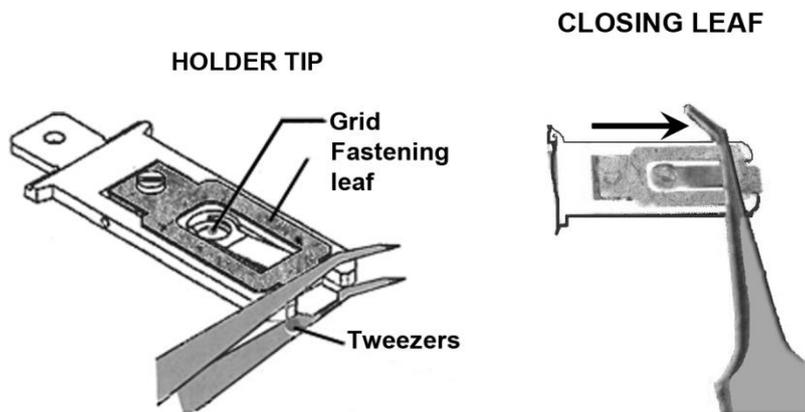
12. Remove any forgotten/left grid from the specimen retainer. Place a new grid with the observation side facing upward in the retainer.
