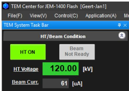
8. If vacuum or HT are not ready, the HT icon on the screen will appear in gray. You can try to switch on the HT by a double click on the icon. The HT should start to raise. **Wait until HT voltage is 120 kV.** If the HT does not reply, warn Geert-Jan
