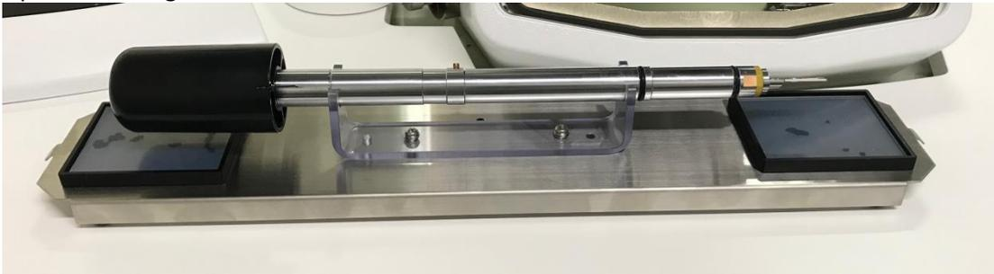
11. To load the grid on the specimen (=sample) holder, clutch the top and bottom of the specimen fastening leaf spring at its clip end from front with a pair of tweezers. The lip will open.
