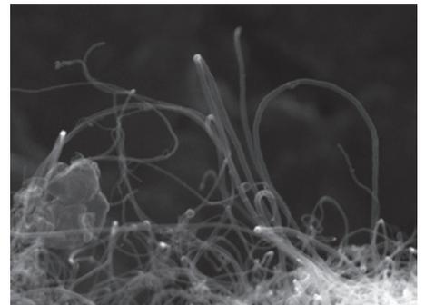
Specimen: Carbon nanotubes
