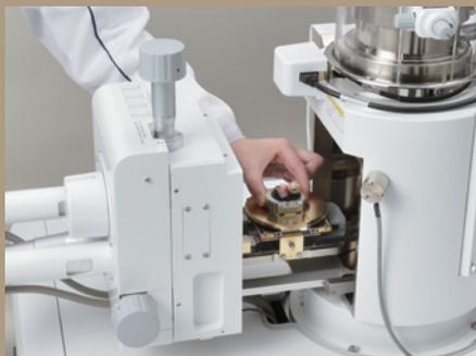
Maximum specimen diameter: 150 mm dia.
