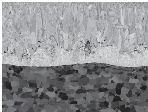
Specimen: Hot dip galvanizing on iron
