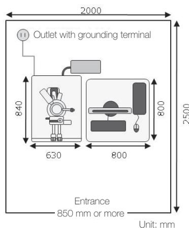
**EDS** Applicable to two configurations: (A) Analysis and (LA) Low Vacuum & Analysis.
