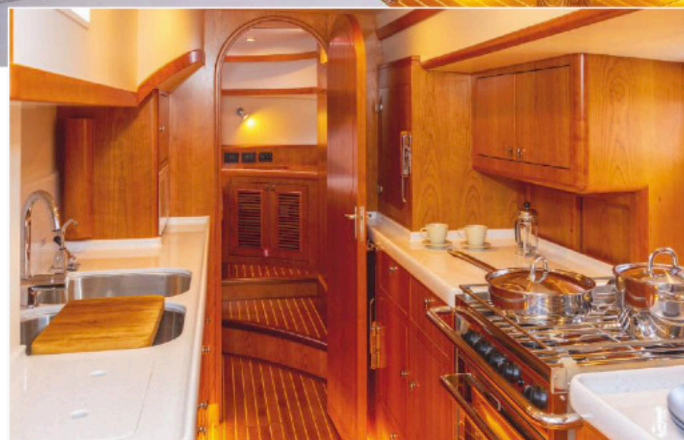
A practical sea-going galley with front-opening fridge and freezer, three-burner cooker, two enormous sinks, special provision for gutting fish, stacks of stowage and a practical gash bin
