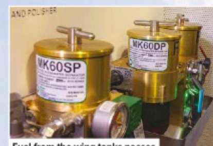
Fuel from the wing tanks passes through two fuel polishing systems as well as the engine's filters
