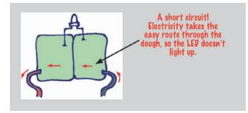
If your two pieces of conductive dough are touching at all, the electricity will flow through the dough, not the LED. This is called a short circuit and may lead to your batteries overheating.
