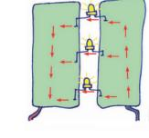
In a parallel circuit, the electricity can take several paths. This means each bulb gets the same amount of electricity and will have equal brightness.
