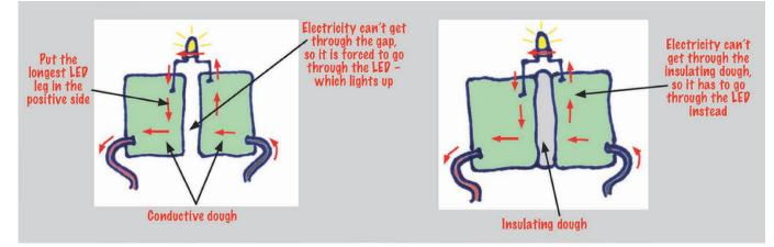
Now try to create a circuit where the insulating dough stops the electricity from travelling anywhere apart from through the LED.
