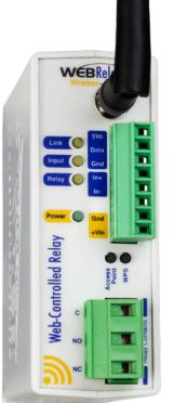
The WebRelay Wireless™ is an easy to use Wi-Fi enabled relay, temperature monitor and status alerting device. The WebRelay Wireless has a built-in relay for controlling lights, motors and other relatively high current loads, a digital input which can be used to monitor and report the status of switch-closure sensors and a "1-Wire" port for connecting up to four digital temperature or other Xytronix 1-wire sensors.
