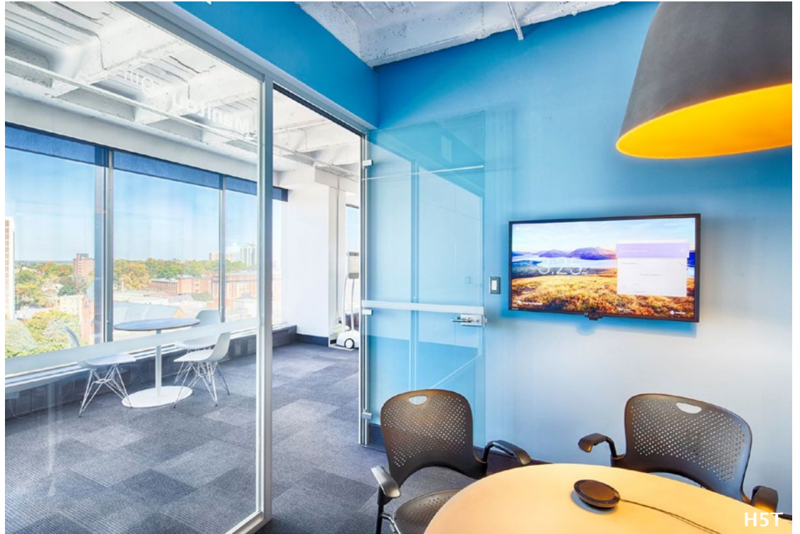
Frame: Full-height glass panels encased in vertical aluminum extrusions
