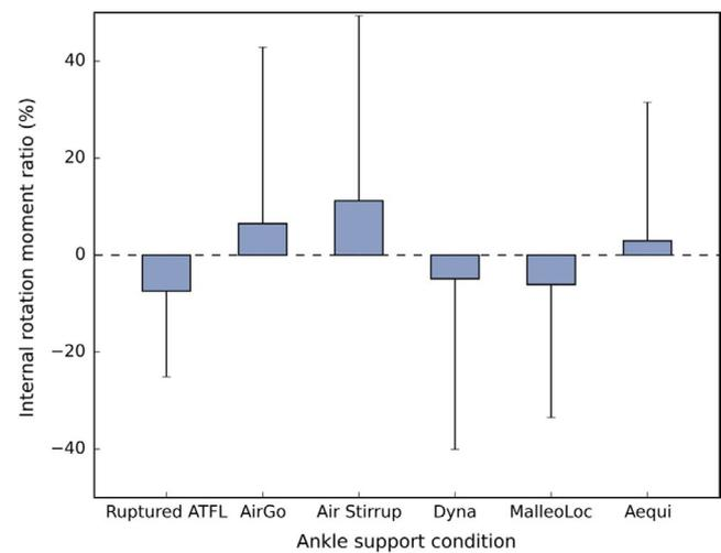
**FIGURE 3** Internal rotation ratios as a function of the stabilizing condition. The baseline represents the intact unprotected state. Loading was applied in dynamic mode at 50°/s. Values are presented in mean ± SD
