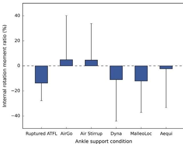
**FIGURE 2** Internal rotation moment ratios as a function of the stabilizing condition. The baseline represents the intact unprotected state. Loading was applied in quasi-static mode at 0.5°/s. Values are presented in mean ± SD
