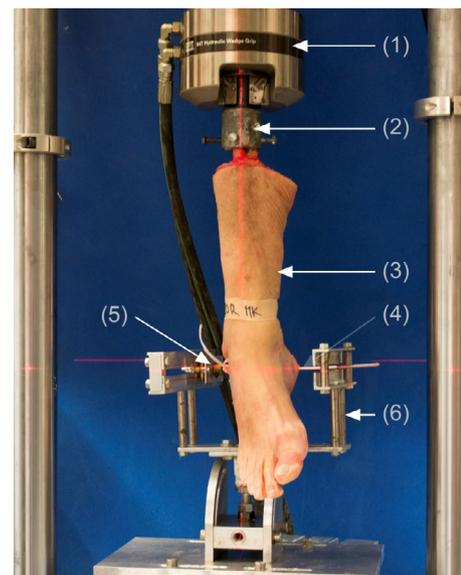
**FIGURE 1** Biomechanical tests were carried out in a hydraulic load frame (1). Using custom-made steel cups (2) and Wood's metal specimens (3) were fixed proximally. The correct alignment was controlled with a laser beam. A Steinmann pin (4) was drilled through the calcaneus and allowed locking in the guide block (5) of the mounting platform (6)
