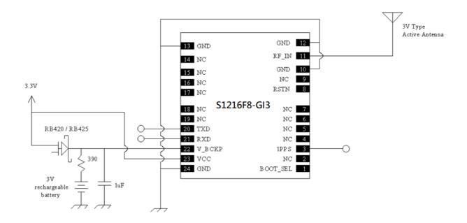
When S1216F8-GI3 has previously been used within 2 hour, for faster time to first fix powering up without needing to decoded ephemeris data from signal, V\_BCKP should be connected to non-volatile supply; above figure with V\_BCKP connected to rechargeable battery is an example implementation. If cold starting every time powering up is not an issue, V BCKP can be connect to VCC.
