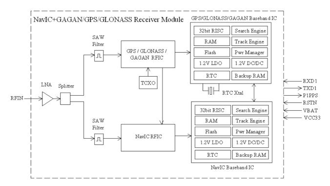
The S1216F8-GI3 is a high performance L5 NavIC + L1 GAGAN/GPS/GLONASS satellite navigation receiver in a compact surface mount package. It is based on the SkyTraq Venus 8 positioning technology, providing high performance signal acquisition and tracking. The simple UART serial interface and the standard NMEA-0183 protocol make usage of S1216F8-GI3 very easy and straightforward.
