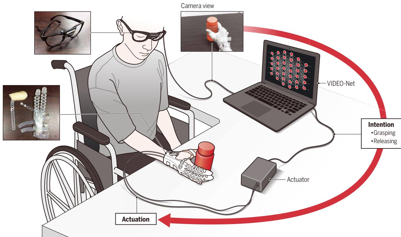
**Fig. 1. System overview.** Our system comprises the wearable hand robot with an actuation system and a computing device, which enumerates “intention” outputs from VIDEO-Net. Exo-Glove Poly is used for the wearable hand robot, and a first-person-view camera is mounted on the glasses. The glove is manipulated by tendon-driven actuators in the actuation system.
