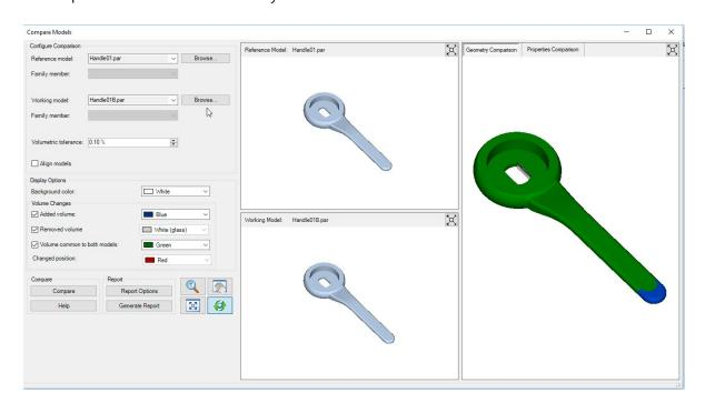
Once it has finished, it highlights the added material in blue and the removed material in a white glass colour.
