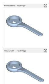
In the Compare Models dialog box, select the Reference Model and the Working Model by selecting the Browse button to select the 2 files. The working model is compared to the reference model.
