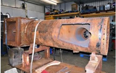
This photo shows part of the lower section of the boiler cut out ready for the metal thickness to be measured in various places. From this a patch of the correct size will be made and welded in place.
